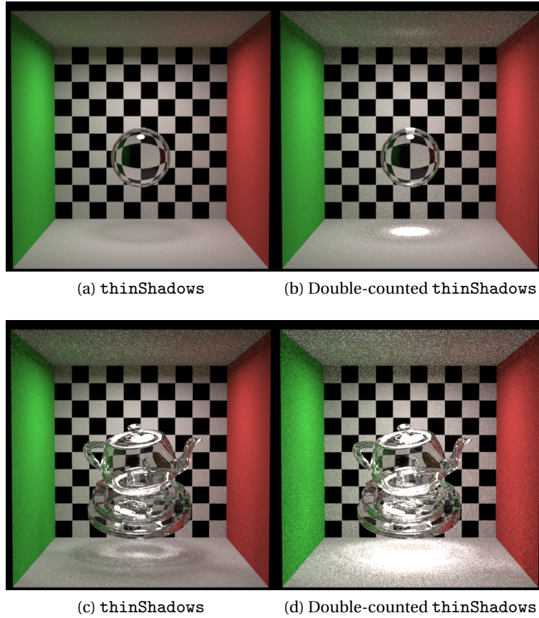
Figure 20: Thin shadows with correct energy (a & c), incorrectly double-counted energy (b & d).
