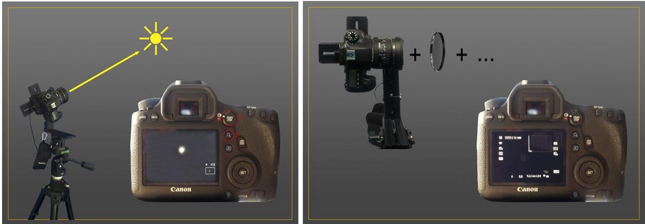
Figure 47: Left: Camera facing the light source. Right: Different filters are installed until the bright light source disappears.
