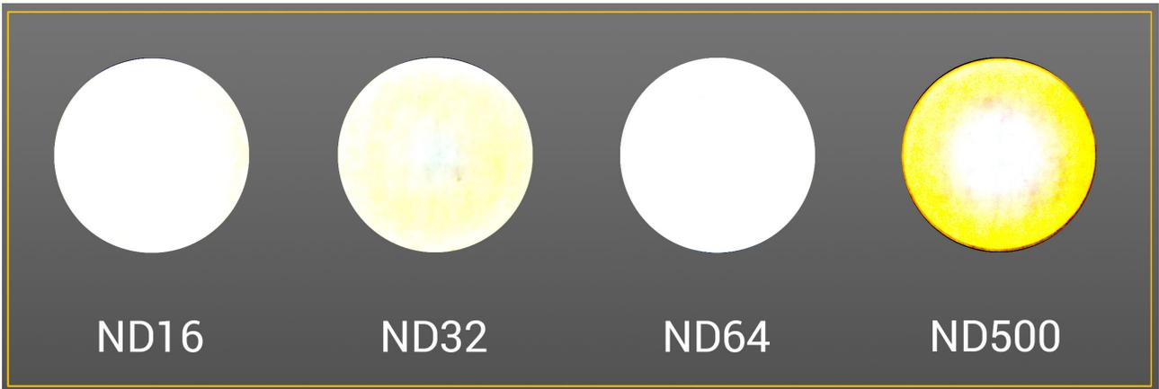
Figure 69: Characterization of various Hoya ND filters. The image is displayed with a range remapping of [0.9 .. 1.0] to [0 .. 1]. This means that only the attenuation from 0.9 to 1.0 is shown. The image shows that vignetting is barely visible and can be ignored. A very slight shift in blue is visible on the ND32 and ND500 (the yellow pattern).
