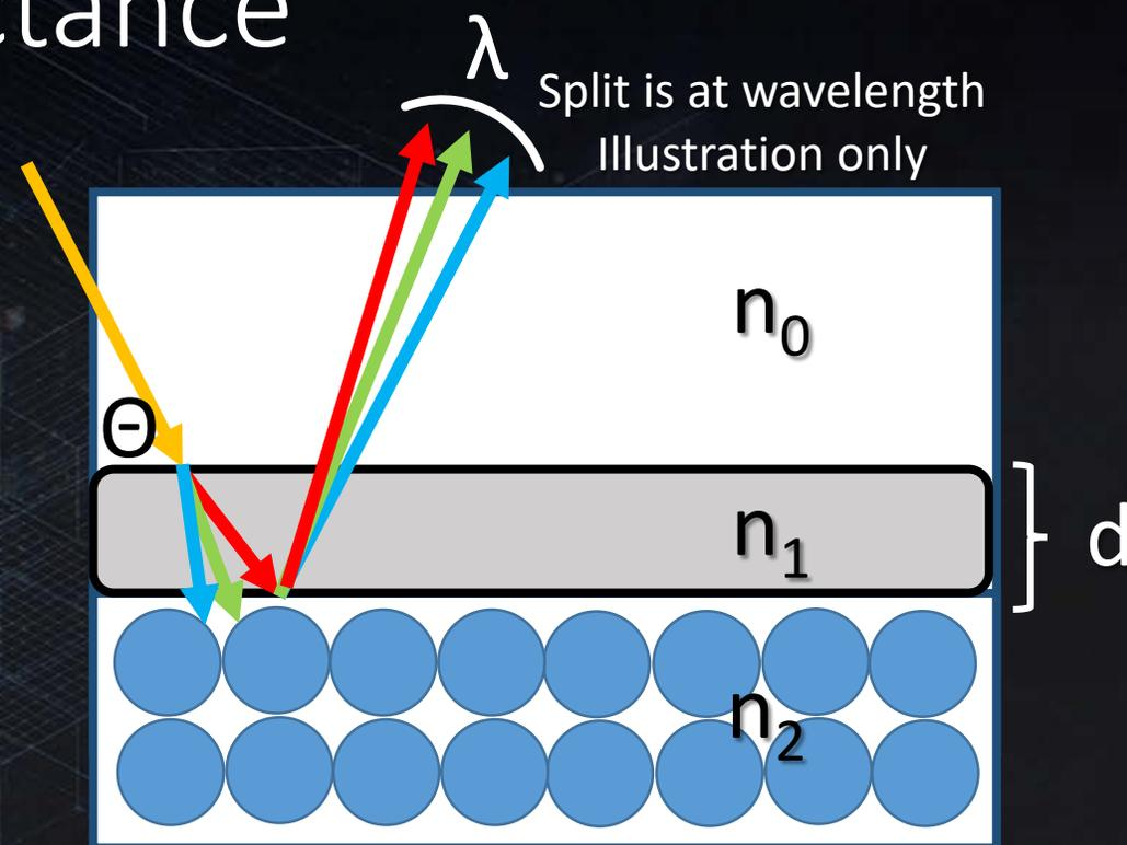
$$s_{i,j} = \text{Fresnel}R_s(n_i, n_j, \theta) \quad \delta = 4\pi \cos(\theta_{\text{transmitted}}) * n_1 * d / \lambda \quad p_{i,j} = \text{Fresnel}R_p(n_i, n_j, \theta)$$
