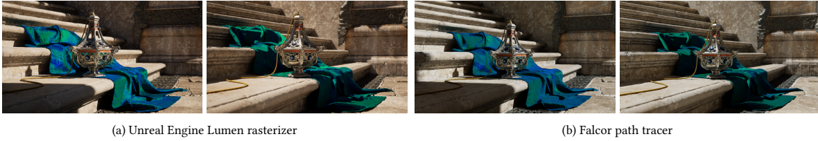
Figure 6: The same asset rendered in a rasterizer and a path tracer, with two different lighting directions. Note that the remaining differences lie in the light transport – particularly indirect bounces, which are handled quite differently.
