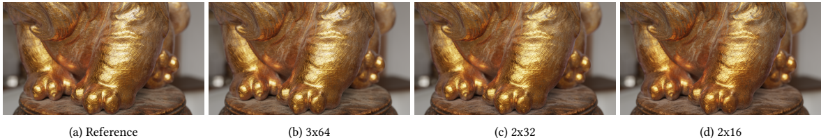
Figure 2: The decoder size will influence performance and quality. While the quality goes down with smaller configurations (in particular the 2x16 version loses some of the color at grazing angles), performance improves. The render time for the reference image is 7.03 ms and goes down to 5.78 ms, 2.69 ms and 1.97 ms for the respective sizes. Model and textures created by Alex Liu and Zhelong Xu.
